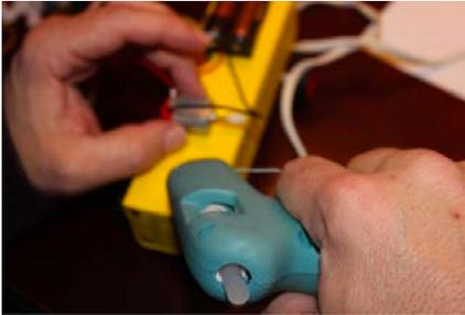
4. Do the same for the battery pack and switch. Make sure the glue has hardened.
