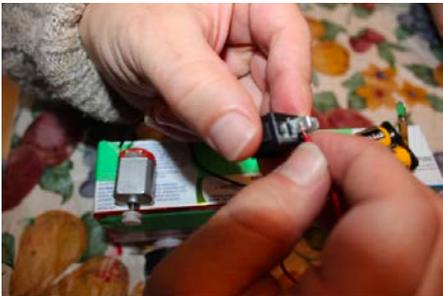
4. Take your small gauge lead wire and strip the ends to expose the copper. You can do this by using wire strippers, scissors, or a knife. Be careful not to cut the copper wires inside when taking the outer sheath off. Note – make sure to strip enough of the sheath off so that it can go through the attachment holes.
