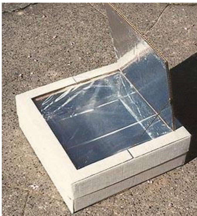
A solar cooker uses an insulated box and reflective panels to generate the temperatures needed to cook food. Photo courtesy of The Solar Cooking Archive
