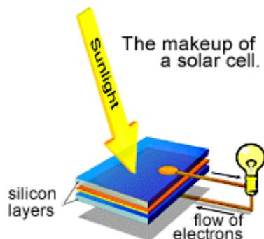
Solar cells are often used in locations where there isn't any electricity and where electricity is needed in small amounts. In such cases, solar cells are usually connected to batteries, allowing electricity to be stored for use during times when the sun isn't shining.
