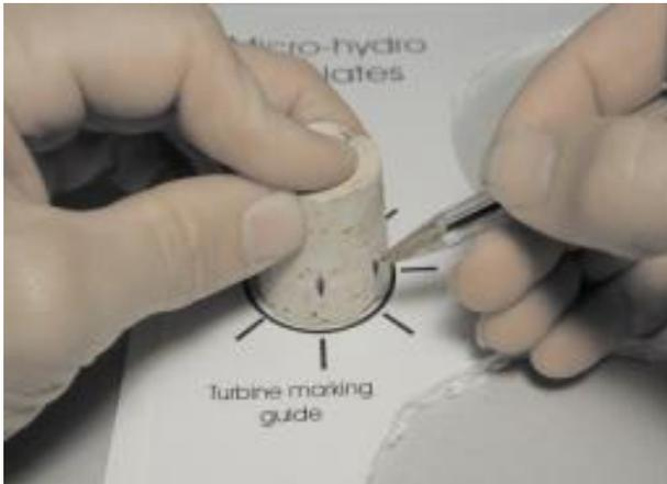
2. Center the wide end of the cork on the marking guide on the template page, and mark the cork with a pen or pencil.
