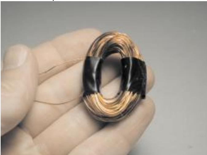
5. Using a small patch of emery cloth or sand paper, remove the enamel insulation from the ends of each lead, exposing about 1 cm of bare wire. Be sure the wire is completely bare!
