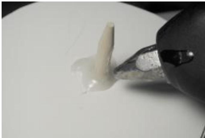
Reinforce the rotor disk with hot glue.
