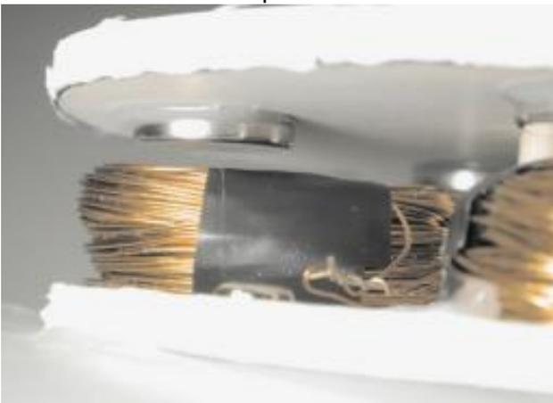
The magnets should be close to, but not touching the coils as they turn.
