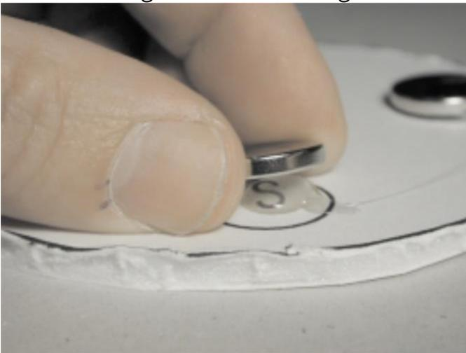
4. Repeat this for the remaining 3 magnets, making sure to alternate north and south poles as you go.
