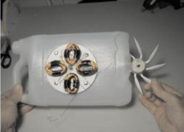
4. Push the shaft through the turbine's cork. Work the cork and the tubing down the shaft so the shaft comes out the other side of the container and projects by about 4cm.
