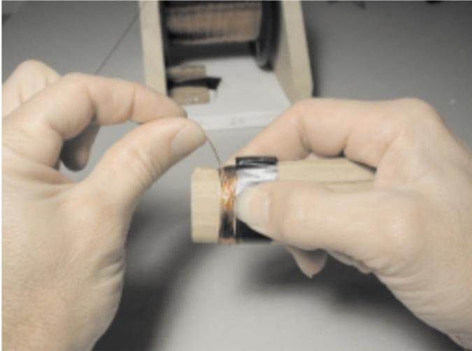
4. Carefully slip the coil off the jig and secure it using two pieces of the electrical tape you set aside in step 2 above.
