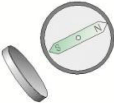
Checking the polarity of one face of a magnet using a compass
