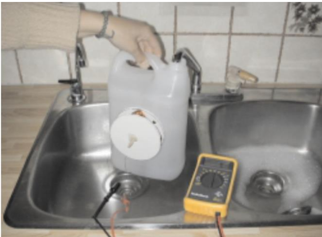
Reinforce the rotor disk with hot glue.
