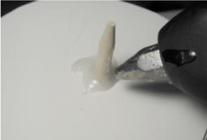
Reinforce the rotor disk with hot glue.
