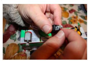
**Step 4:**Take your small gauge lead wire and strip the ends to expose the copper. You can do this by using wire strippers, scissors, or a knife. Be careful not to cut the copper wires inside when taking the outer sheath off.
