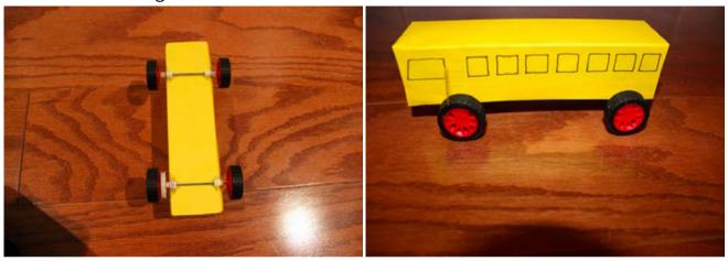
*Tip:* Consider the weight of your electric vehicle while making this part. It it's lighter, you can use a small pulley on the motor to make the car go faster. If the car is heavier, you will need to put the elastic directly on the shaft of the motor. The weight of the car depends on your pulley ratio between your axle pulley and motor pulley. Think of the way the gearing ratio works on a bicycle.
