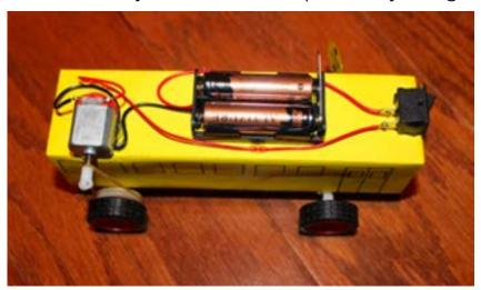
**Step 6:** Voila! Your electric vehicle is finished! You may want to have one learner on the opposite end to catch the vehicle as you race them. Turn the switch on and watch it go! If you are using rear wheel drive, you may want to pick up the rear axle and then turn the power on so that the wheels don't run away from you.
