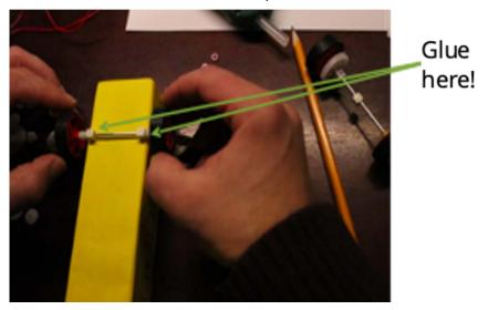
**Step 3:** Place two large dabs of hot flue near the edges of the electric vehicle body. While it is hot, place the two cylinders into the hot glue. Press down firmly for a few seconds while the glue cools.
