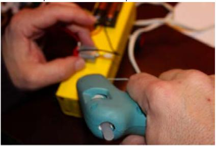
**Step 4:** Do the same for the battery pack and switch. Make sure the glue has hardened.
