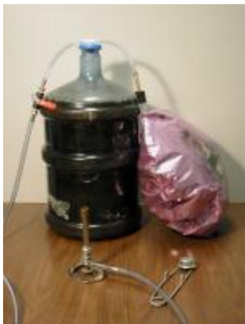
Completed biogas generator
