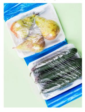
Low-Density Polyethylene (LDPE) "is a softer, clearer, more flexible version of HDPE—and it has its own strengths as well. It's often used as a liner inside juice and milk cartons, and it's used in corrosion-resistant work surfaces and other products, such as six-pack rings and plastic wrap" (Plastics Industry Association, 2021).
