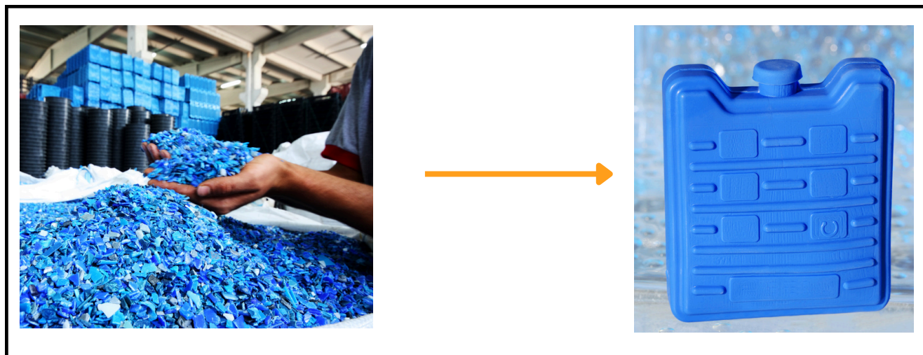
Example of blue plastic pellets being molded into an ice pack.
